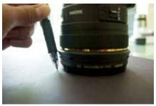
1. Cut and shape the sheet to make a fake lens hood. The Diameter is made so that it snugly fits on the lens. Get a pencil or pen and trace around the lens with the pen abutting the side of the lens.
